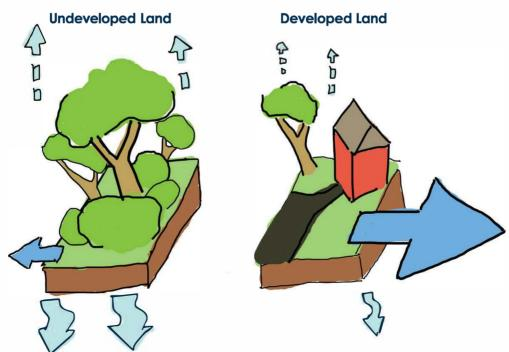
When it rains on an undeveloped piece of property, much of the rainwater infiltrates into the soil or is evapotranspired back into the atmosphere. When vegetation is replaced with streets, driveways, sidewalks, houses, and lawns, less rainwater is able to infiltrate or return to the atmosphere, and more of the rain turns into runoff.
