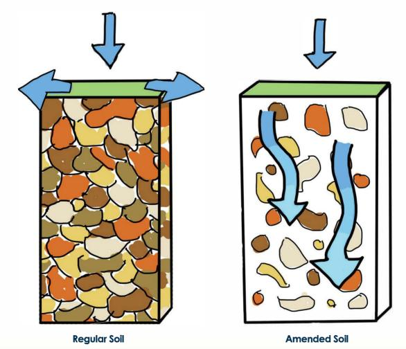
There needs be air spaces in between soil particles for water to be infiltrated. Amended soils have increased air space, but these air spaces are lost if the soil is compacted by heavy equipment or vehicle parking.
